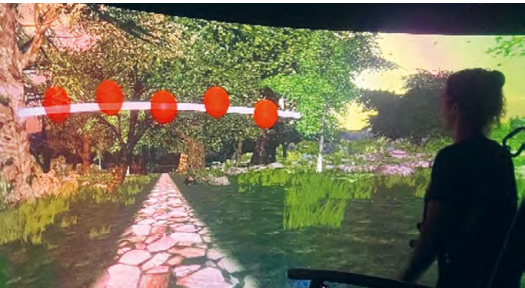
Virtual reality treadmill training. Left: Setup with treadmill, screen with integrated visual feedback for patients, cameras for precise movement analysis, and a control panel. Right: Visual feedback for patients – the white line indicates the target value of the selected gait parameter, while the red dots display the current measurements during training.
